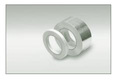
FT-1L...fixing tapes for circumferential banding cable to piping every 30 cm or as required by code or specification. AL-20P...aluminium tapes for continuous (longitudinal) covering and/or circumferential banding cable to piping and/or equipment.
