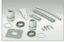
**PETK-SXM-OJ-IND...**circuit fabrication kit terminates SX heating cables in a JB-K-1 (or other) junction box. Kitincludes an M25 tracer gland (with locknut), power boot, end cap, RTV adhesive, yellow/green earth wire sleeve, the necessary wire pins/lugs plus an insulation entry kit.
