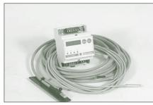
**DHB 350..** ice-control, 230 Vac, 13A consisting of a combined control unit with humidity and temperature probe. The control unit switches the heating cable on when the ambient temperature is below 3 deg. C, and icy water/snow is present in the gutter.
